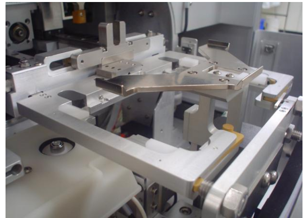
Figure 2. Mono-Lift nest ready to receive a plate into the destination gripper of an ATS.
